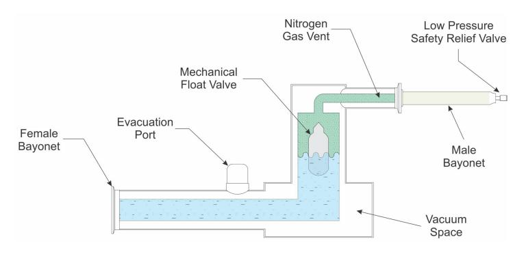
Gas Vents remove excess gas from the system to maintain liquid level and provide liquid on demand after a shut down period.
